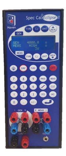
The Spec-Cal® Eclipse II measures and simulates 12 thermocouple types to any of four selectable international standards (BS, JIS, DIN and ANSI) as well as simultaneously measuring or generating mV, mA or Volts. In addition, the Spec-Cal® Eclipse II measures and generates ohms, and measures and simulates 7 different RTD types.
